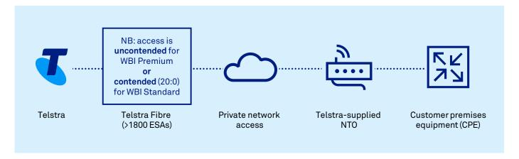
The Telstra Wholesale Business Internet™ NTU is the segregation point. The customer CPE connects to Telstra's internet network by a gateway to provide private network access utilising Telstra fibre.
