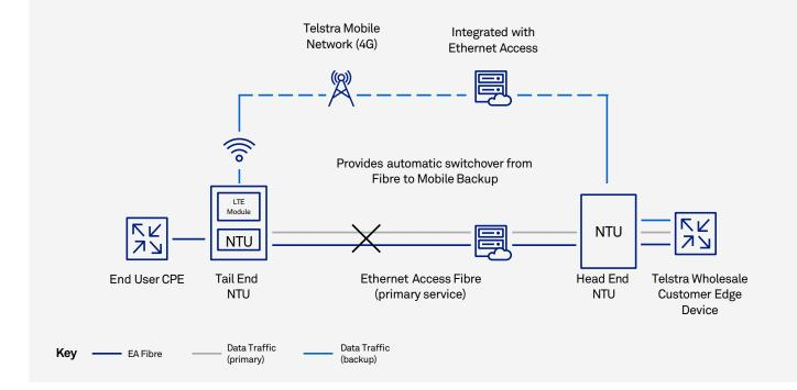
Mobile Backup automatically provides connectivity if the tail-end Ethernet Access fibre goes down. Your customers stay connected.
