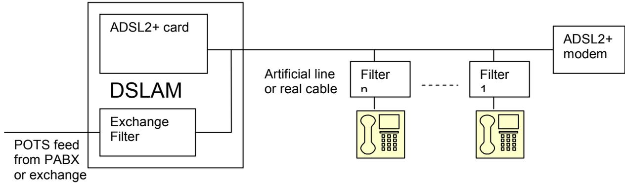
**Figure 4 – Test layout for POTS compatibility testing (note: for central filter use one filter and 3 telephones)**
