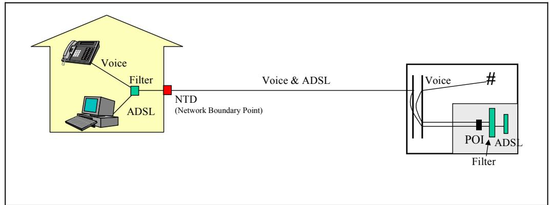
**Figure 1 – Telstra Wholesale Spectrum Sharing Service (End-to-End View)**
