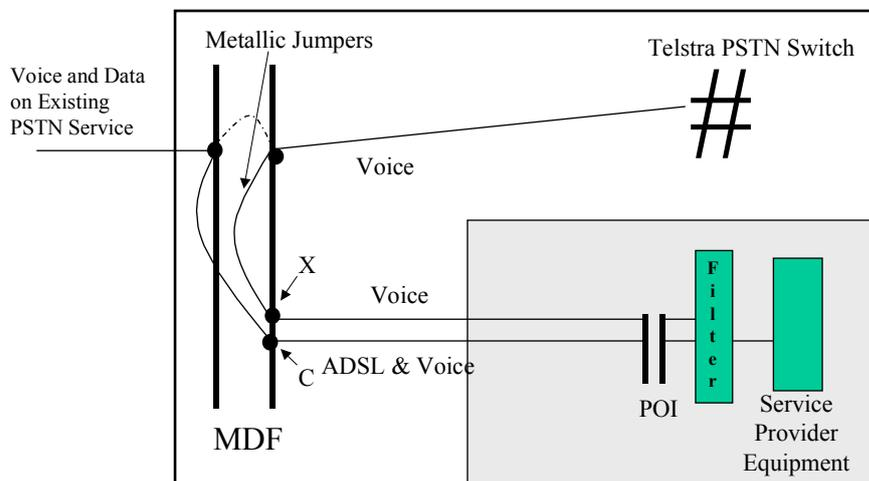
**Figure 2 – Telstra Wholesale Spectrum Sharing Service (Voice provided by Telstra, ADSL provided by Acquirer)**
