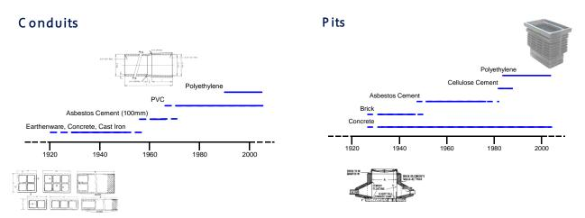
Many fibre cement pits are likely to contain ACM and as such, Telstra applies the presumptive test that all non-plastic pits and pipes/conduits/ducts are to be treated as ACM. Older suburbs adjacent to modern CBD areas are likely to have a larger number of pits and pipe/conduit/ducts that are likely to contain ACM.
