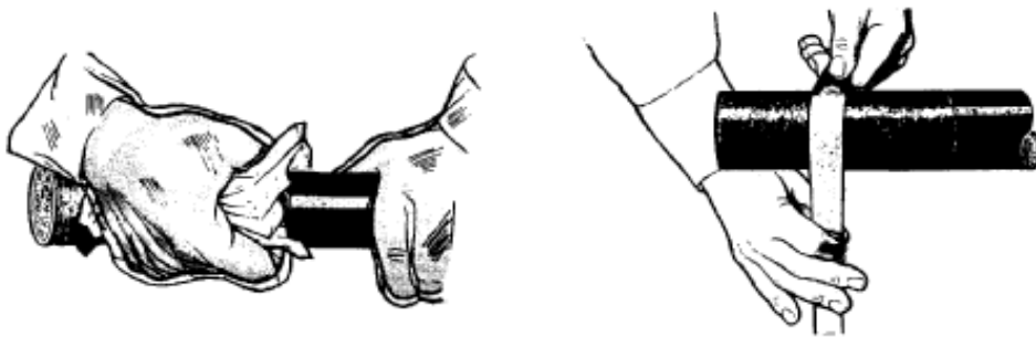
Figure 6 - Cleaning and abrading cable sheath
